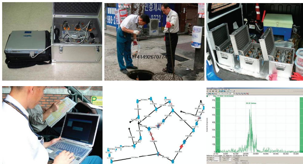
Figure 8. Leak detection using multipoint leak noise correlator [□] (Upper left: leak detection device, upper middle: installing data logger in the valve room, upper right: data collection from the logger, lower left: data analysis, lower middle: symptom of leak (red dots), lower right: leak confirmation through data analysis)
