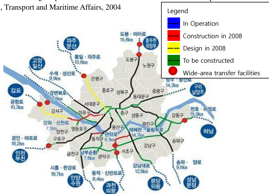
Figure 3: Installation Planning Map of Exclusive Median Bus Lanes in Seoul Metropolitan Government, Ministry of Land, Transport and Maritime Affairs, 2008
